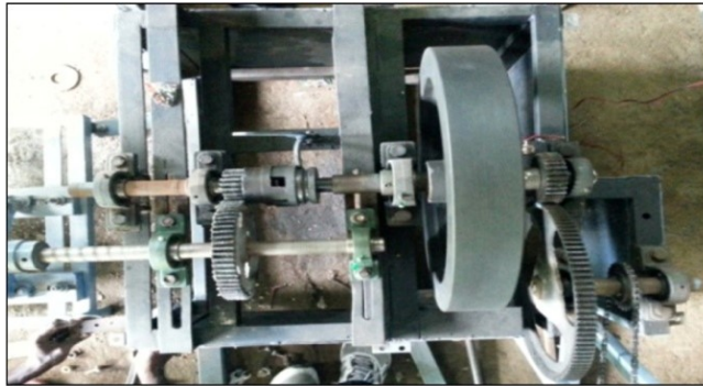
Figure 3: Mechanical power transmission unit.
