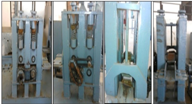
Figure 4: Different views of bamboo sliver cutting unit.
