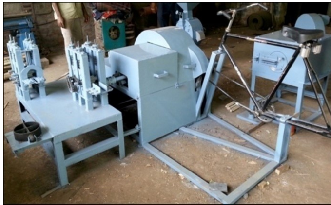
Figure 1: Human powered bamboo slivering machine.
