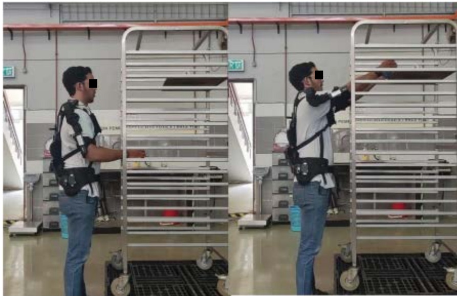
Figure 2: The arms were initially at 0 degree, then elevated to 135 degrees at around head height.
